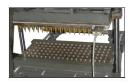
The ZE 50-PN series of semi-automatic machines are used for baking ice cream cones, moulded sugar cone and cups. These machines are easy to use and robust. The heating is by electrical heaters designed to optimize energy use and thermal distribution; This machine is flexible for high production on nonstop basis for 24 hours.
